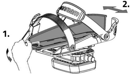
With the axel pedal extender the foot support can be extend further.
