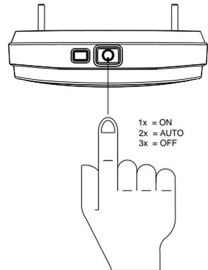
sensors. When the bicycle stands still for a while, the light will automatically turn off.
