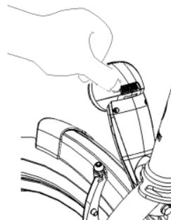
The headlight can be manually switched on or off with the "On/Off" position.
