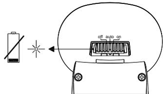
1. Remove the two screws at the back of the front light.
