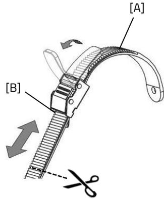
The position of the foot support on the pedal is adjustable in length. This allows you to pedal with the ball of your foot for better thrust.
