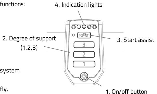
After the system is turned on, the electric motor is active in level 1.
