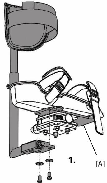
2. Adjust the height of the lower leg support in such a way that it is aligned with the lower leg of the rider.
