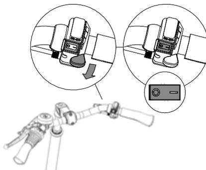
There is no option to change the maximum speed in the reverse mode. The LED lights of the support levels 1, 2 and 3 burn to indicate that the reverse mode is activated.
