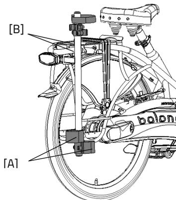
To use the flashing lights press the switch [A] to the left or right. To turn off the indicators, move the switch to the centre position.
