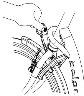
In the "Auto" position, the headlight turns on or off automatically with the help of light- and movement sensors. When the bicycle stands still for a while, the light will automatically turn off.
