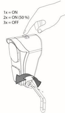
The headlight is powered by batteries. When the batteries are nearly empty, the LED light in the button of the headlight will turn red. Follow the steps to change the batteries of the headlight.
