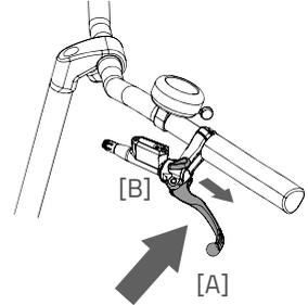
To operate the parking brake, squeeze the left brake [A] and secure the brake with the lever [B].
