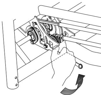
To keep the tension of the two chains at the front correct, you can adjust the special tension wheels by the pedal axes. To do this:
