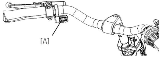
If you want to switch off the flashing light system, put the switch in the middle position.
