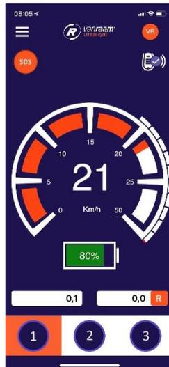
This app can be used as a luxury bicycle computer for Van Raam bicycles with pedal assistance and also contains many other extra functionalities. The dashboard on the app shows the current speed, total distance, trip meter, battery capacity and power consumption during the bike ride. For more cycling data, there is a details screen including average speed, maximum speed, total distance, power, battery voltage, pedaling power and pedaling frequency.
