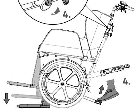
6. To lift the footrest, place your foot on the control pedal and **slowly** press the pedal down until it locks and you can hear a 'click'.
