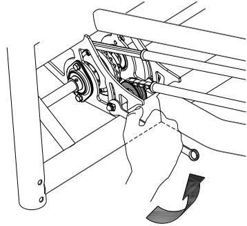
To keep the tension of the two chains at the front correct, you can adjust the special tension wheels by the pedal axes. To do this:
