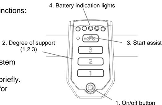
After the system is turned on, the electric motor is active in level 1.
