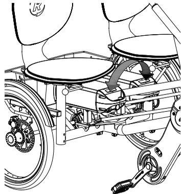
One of the battery holders is connected to the system, you can recognize this one because of the cables.
