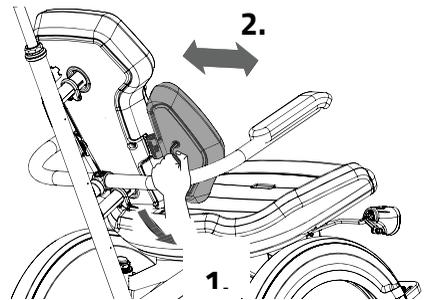
Finish by adjusting the angle of the side supports.
