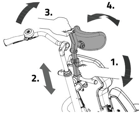
**Please note:** make sure the handlebars can easily move after setting up the headrest.
