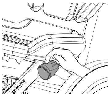
By pressing the pressure switch once, the front light will turn on. By pressing again the lamp will switch to 'Auto' mode (a green LED will flash for 5 minutes). Finally, a third press will turn the front light off.
