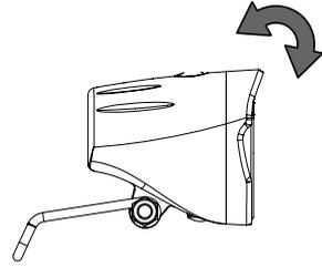
Adjust the angle of the headlight, so that the centre of the light beam is aimed about ten metres in front of the bike.
