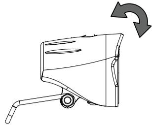
Under the pressure switch on the top of the front light is a battery indicator that lights up when the batteries are low. Once the battery indicator starts lighting up red, replace the batteries as soon as possible.
