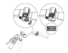
There is no option to change the maximum speed in the reverse mode. The LED lights of the support levels 1,2 and 3 burn to indicate that the reverse mode is activated.
