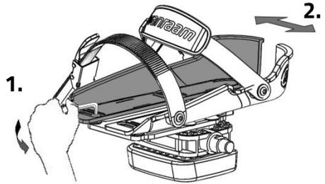
With the axel pedal extender the foot support can be extend further.
