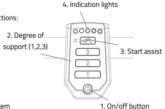
After the system is turned on, the electric motor is active in level 1.
