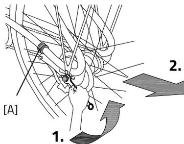
3. At the same time make sure that the wheel is straight and positioned in the centre of the frame, as illustrated. Not to the left or to the right.
