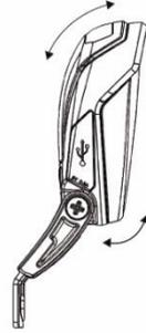
Adjust the angle of the headlight, so that the centre of the light beam is aimed about ten metres in front of the bike.
