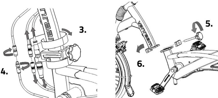
To assemble the tricycle again, follow these steps in reverse order. When connecting the cables, make sure that the arrows or cams are directly opposite to each other.
