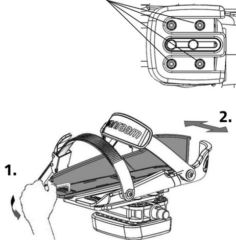
With the axel pedal extender the foot support can be extend further.
