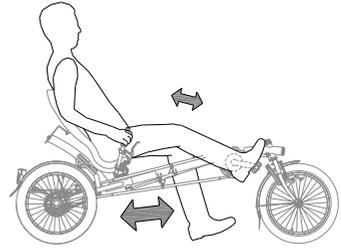
The saddle position is adjusted by shifting the frame length to the right distance.
