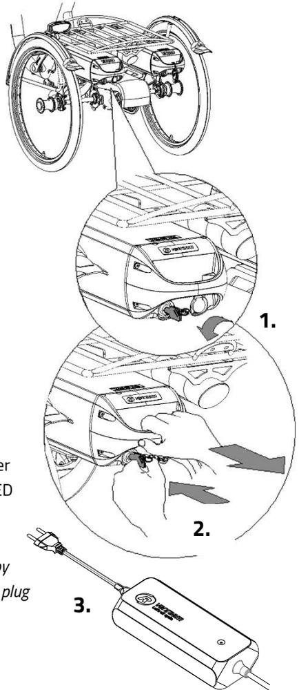
5. The charging time depends on the level of the battery. The charging time is about 2 hours for a 10.7 Ah and about 4,5 hours for a 24.8 Ah battery.
