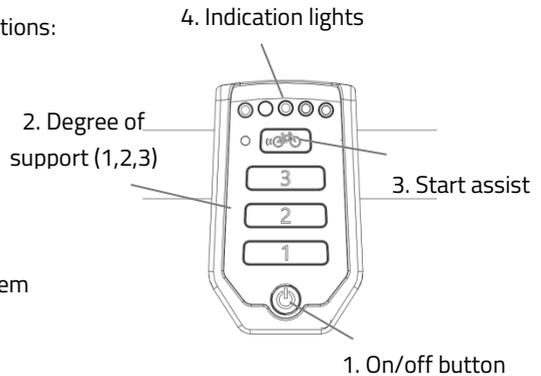
After the system is turned on, the electric motor is active in level 1.
