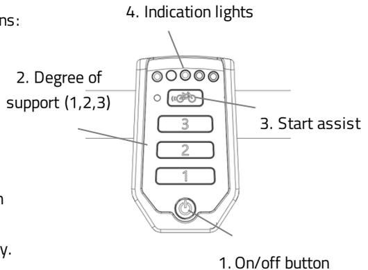
After the system is turned on, the electric motor is active in level 1.
