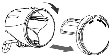
3. Replace the alkaline batteries (1.5 V - 1500 mA) and reattach the front cover.
