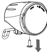
2. Remove the front cover by turning it slightly and pulling it forward.
