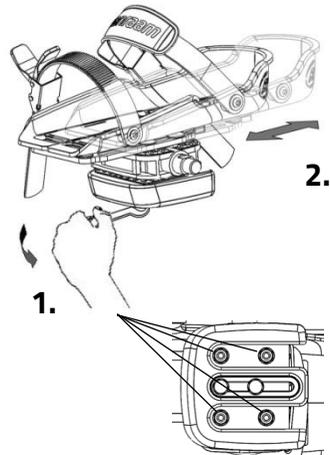
The foot support is also adjustable in width. Only the outer half of the foot support can be extended.
