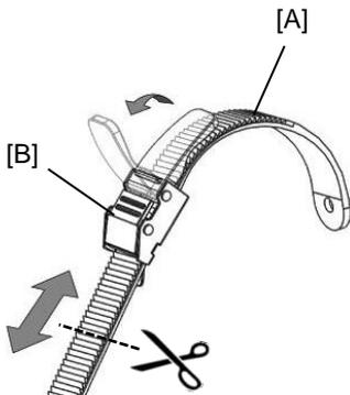
The position of the foot support on the pedal is adjustable in length. This allows you to pedal with the ball of your foot for better thrust.
