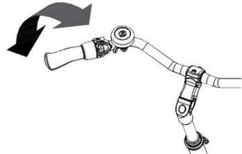
When steering from the rear, there is a third position. In that position the pedals of the co-driver move independently of the pedals of the main driver. The co-driver can cycle along independently.
