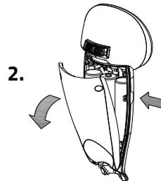
3. Replace the alkaline batteries (1.5 V - 1500 mA) and assemble the rear cover.
