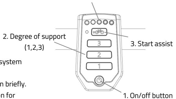
After the system is turned on, the electric motor is active in level 1.
