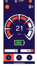
power consumption during the bike ride. For more cycling data, there is a details screen including average speed, maximum speed, total distance, power, battery voltage, pedaling power and pedaling frequency.
