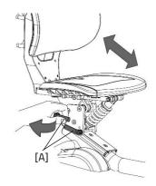
**Caution!** Make sure the quick-release levers have the correct tension to ensure they are properly clamped in place.
