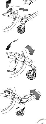
User manual O-Pair² 16.05 4. There is another alternative for adjustment if it is not possible for these adjustments to find the correct position. The foot support can be mounted one hole to the front or one hole to the back. To do this: Loosen the screws completely with a socket wrench and move the foot support to the desired position. Tighten the screws again.
