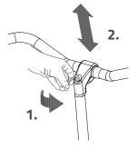
Do not **slide the** handlebars stem further than the markings. If you do so, the tube won't be inserted deep enough into the shaft, increasing the risk of breakage, which may lead to serious injuries.
