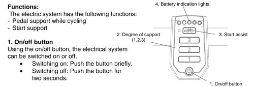
After the system is turned on, the electric motor is active in level 1.
