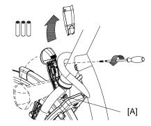
Dismantle the rear cover by pressing with the thumb and index finger at the cavity on both sides of the front cover and pulling the rear cover back.
