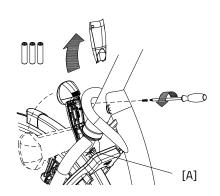
2. Dismantle the rear cover by pressing with the thumb and index finger at the cavity on both sides of the front cover and pulling the rear cover back.
