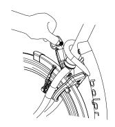
In the "Auto" position, the headlight turns on or off automatically with the help of light- and movement sensors. When the bicycle stands still for a while, the light will automatically turn off.
