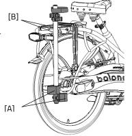
To use the flashing lights press the switch [A] to the left or right. To turn off the indicators, move the switch to the centre position.
