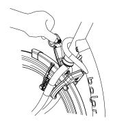
In the "Auto" position, the headlight turns on or off automatically with the help of light- and movement sensors. When the bicycle stands still for a while, the light will automatically turn off.
