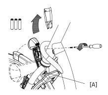
2. Dismantle the rear cover by pressing with the thumb and index finger at the cavity on both sides of the front cover and pulling the rear cover back.
