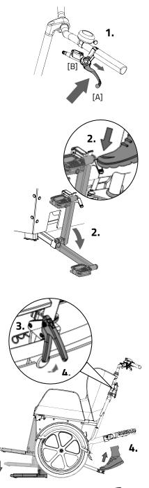
To lift the footrest, place your foot on the control pedal and **slowly** press the pedal down until it locks and you can hear a 'click'.
