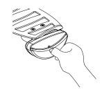
The front light works on the dynamo. Push the button so that the dynamo moves against the tyre. To turn off the light push the dynamo back again.
