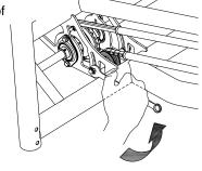
To keep the tension of the two chains at the front correct, you can adjust the special tension wheels by the pedal axes. To do this:
