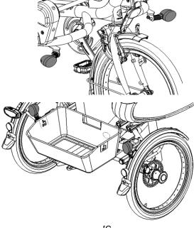
The lights work on a battery. To replace the batteries, turn the screw on the cap and take the orange cap [B] away. Then remove the PCB [C] from the holder. You can now replace the battery [D].
