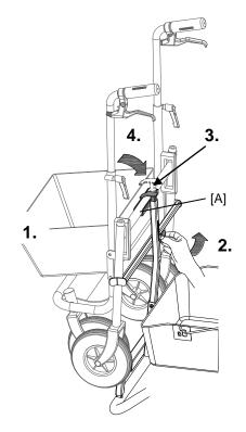
To disassemble the rack, all screws can be loosened with an Allan key. Once they are loosened, all the pipes can be taken out of the frame.
