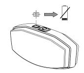
Dismantle the cover of the holder by pressing in the lip at the bottom of the light.
