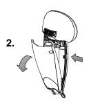
3. Replace the alkaline batteries (1.5 V - 1500 mA) and assemble the rear cover.
