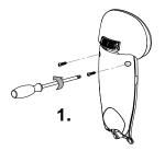
Dismantle the rear cover by pressing with the thumb and index finger at the cavity on both sides of the front cover and pulling the rear cover back.
