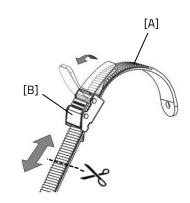
The position of the foot support on the pedal is adjustable in length. This allows you to pedal with the ball of your foot for better thrust.
