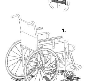
Loosen the screws with an Allen key to adjust the supports.
