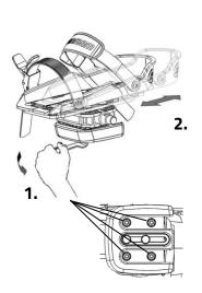
The foot support is also adjustable in width. Only the outer half of the foot support can be extended.
