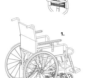
Loosen the screws with an Allen key to adjust the supports.
