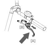
To operate the parking brake, squeeze the left brake [A] and secure the brake with the lever [B].
