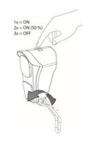
The headlight is powered by batteries. When the batteries are nearly empty, the LED light in the button of the headlight will turn red. Follow the steps to change the batteries of the headlight.
