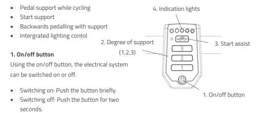
After the system is turned on, the electric motor is active in level 1.
