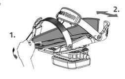
With the axel pedal extender the foot support can be extend further.
