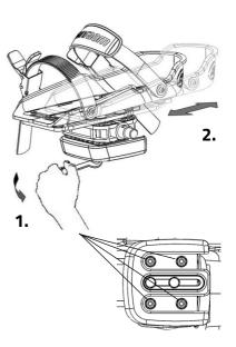
The foot support is also adjustable in width. Only the outer half of the foot support can be extended.
