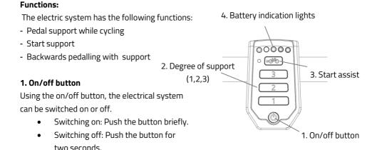
After the system is turned on, the electric motor is active in level 1.
