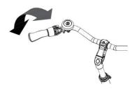
When steering from the rear, there is a third position. In that position the pedals of the codriver move independently of the pedals of the main driver. The co-driver can cycle along independently.
