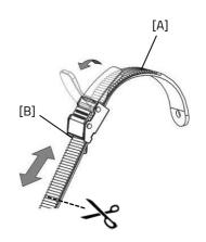
The position of the foot support on the pedal is adjustable in length. This allows you to pedal with the ball of your foot for better thrust.
