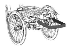
Both battery holders are connected to the system, you can recognize this because of the cables.
