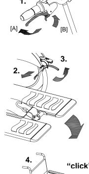
**Be sure** that the ramp is locking! Failing to do so may result in serious injuries. If the ramp does not lock properly then use your foot [A] to push until the ramp locks.
