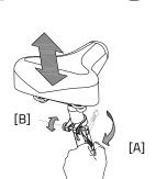
Don't **pull out** the seat post further than the markings. If you do so, the tube won't be inserted deep enough into the shaft, increasing the risk of breakage, which may lead to serious injuries.
