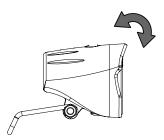
Adjust the angle of the headlamp. Make sure that the centre of the beam is approximately ten meters in front of the bike.
