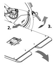
Make sure that once the wheelchair is placed on the ramp, the wheelchair's weight causes the ramp to fold up automatically. When that is the case, the centre of gravity of the wheelchair is situated above the front wheels of the bicycle. This creates the correct weight distribution of the bicycle.
