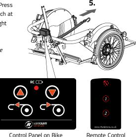
Position the wheelchair straight in front of the ramp and attach the hook to the wheelchair.
