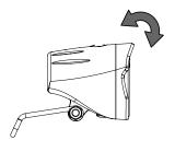
Adjust the angle of the headlight, so that the centre of the light beam is aimed about ten metres in front of the bike.
