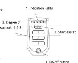
After the system is turned on, the electric motor is active in level 1.
