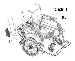
**Please note!** Make sure that the ramp locks into place! Otherwise dangerous situations may arise. If the ramp does not lock in to place, press on it with your foot [A], so it clicks into place.
