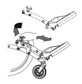
2. There is another alternative for adjustment if it is not possible for these adjustments to find the correct position. Both bracket plates can be mounted one hole to the front or one hole to the back. To do this: Loosen the screws completely with an Allen key and move the plates to the desired position. Tighten the screws again.
