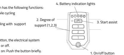
With the option "integrated lighting", the lights will automatically switch on when you turn on the electric motor system. You can switch the lights on and off by briefly pressing the on/off button in this mode.
