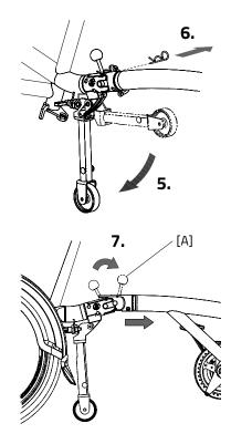
Make sure the wheelchair rests on the front nose wheels when the back frame is attached. As soon as the frame has been attached, the wheelchair section can be titled backwards due to which the connection snaps into place.
