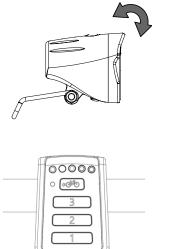
Adjust the angle of the headlight, so that the centre of the light beam is aimed about ten metres in front of the bike.
