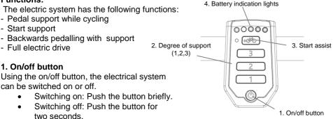
After the system is turned on, the electric motor is active in level 1.
