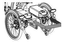
One of the battery holders is connected to the system, you can recognize this one because of the cables.
