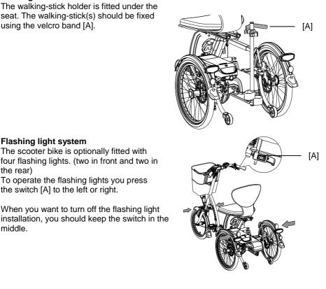
The flashing lights work on batteries. The batteries are present only in the front lights, the rear lights are connected to them.
