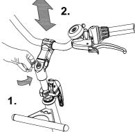
Do not pull out the handlebars further than the mark.
