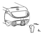
If necessary, the battery can also be charged directly on the cycle.
