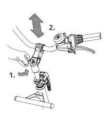
Do **not** pull out the handlebars **further** than the mark. Otherwise the tube will not be deep enough in the shaft and will risk coming off, which can lead to serious injuries.
