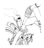
In the "Auto" position, the headlight turns on or off automatically with the help of light- and movement sensors. When the tricycle stands still for a while, the light will automatically turn off.
