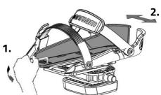
With the axel pedal extender the foot support can be extend further.
