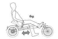
The saddle position is adjusted by shifting the frame length to the right distance.
