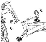
To assemble the tricycle again, follow these steps in reverse order. When connecting the cables, make sure that the arrows or cams are directly opposite to each other.
